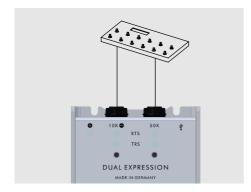
Some multi effects pedals have multiple control inputs for expression pedals. With the LEHLE DUAL EXPRESSION you can use two inputs and by means of the 10K socket trigger the switching function which can use your multi effects pedal on the other hand to, e.g. switch a preset, activating a Wah pedal or whatsoever your effects pedal makes possible.
