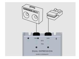
The 10K socket can be used as a momentary or latching switch. This way you can control external devices.
