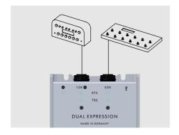
By means of the additional 10K socket as a switching output, it's very easy and flexible to control the KEMPER<sup>™</sup> PROFILER<sup>™</sup> devices. This way you can activate and deactivate, e.g. the Wah pedal or any other effects in the KEMPER<sup>™</sup>.
