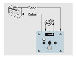
Many amplifiers feature only one serial effects loop, which means that the signal is routed entirely via this loop between the preamp and the power amplifier.
