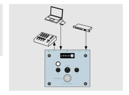
Check the overall sound for any phase cancellations and, if necessary, press the phase reverse switch (4) on the LEHLE PARALLEL SW II.
