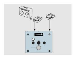
The LEHLE PARALLEL SW II can also be used to mix two different signals.
