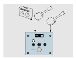
If you connect a mono signal to the input socket (1) and a stereo signal to the return socket (5), please press the monoto-stereo switch (2) too.
