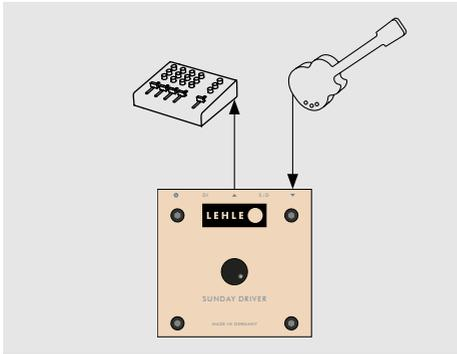
The signals from piezo pickups, like those used on acoustic instruments, are often too weak for the line inputs of a mixer.
