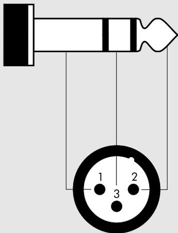
Balanced signal lines are fitted with XLR connectors or TRS (Tip Ring Sleeve) jack plugs. In a balanced signal line, the signal is present in phase at the tip, as in the case of an unbalanced signal line (XLR Pin 2).
