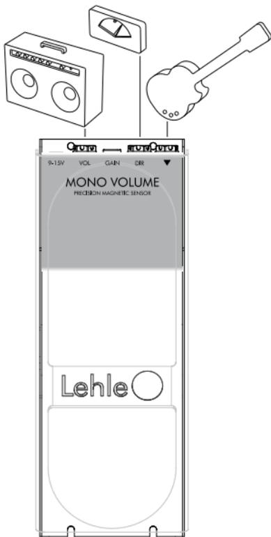
The main purpose of the **Lehle Mono Volume** certainly is adjusting the volume of the connected instrument. The DIR output can be used for a tuner to silently tune the instrument with the VOL output volume turned down. Of course, this output can remain free.
