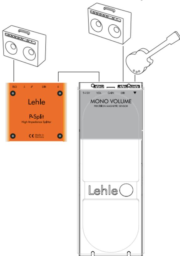
With this setup you can blend your original sound with the sound of a second amp. The amp connected to the DIR out is always on, while the second amp can be faded in and out smoothly via the VOL out. Using the **Lehle P-Split II**, as shown here between the VOL output and the second amplifier is optional. In case ground loops or phase cancellations occur, these will be eliminated effectively by using the **Lehle P-Split II**.
