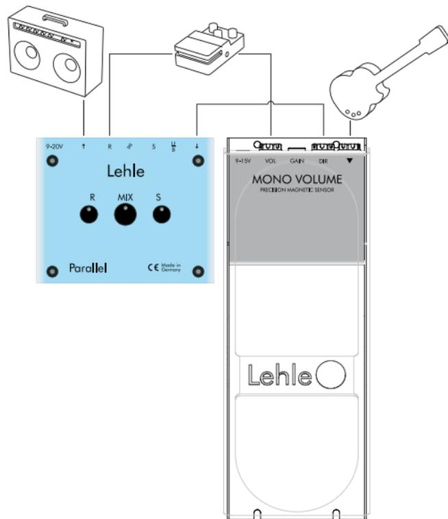
Many effects, like delay, chorus or reverb sound much better when they are blended with the dry instrument signal. This can also be done with the **Lehle Mono Volume**. However, you will need a mixer - in our example, we are using a **Lehle Parallel M**.
