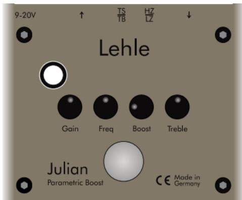
When using acoustic or semi-acoustic instruments you want to avoid feedback in any case, the **Lehle Julian** can help to find and cut the respective feedback frequencies without altering the original sound of your instrument. Turn up the boost controller all the way to the right and start scanning for the loudest point of feedback by using the Freq controller, once you have found it leave the Freq controller in this position and turn the Boost controller to the left until the feedback is gone.
