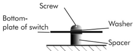
Thanks to its ready-to-go fixing system, the **Lehle Julian** can be mounted without difficulty on a base plate. To do this, undo the four housing screws and detach the cover. Then fix the device base to a base plate using the two screws, the washers and the spacers supplied. Replace the cover and tighten the four housing screws – done!
