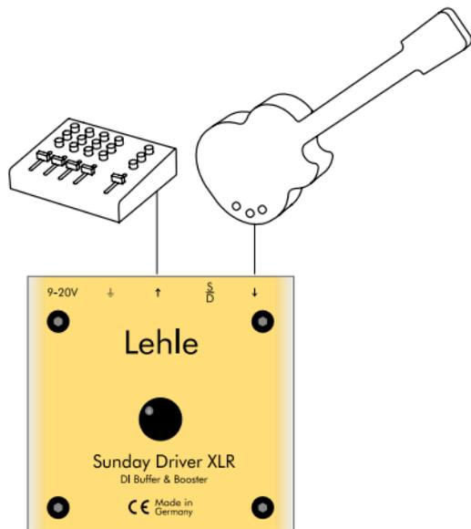
Due to their input impedance of approx. 10 KOhm, the balanced inputs on mixers are not suitable for level-matched recording of high-impedance signals from magnetic pickups (e.g. the single coil and humbucker pickups on guitars and
