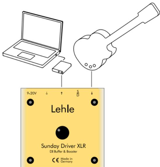
PCs featuring either integrated or external sound cards, and even Digital Audio Workstations (DAWs), often lack the high-impedance instrument input needed for direct recording from an instrument. Connecting the instrument to the standard
